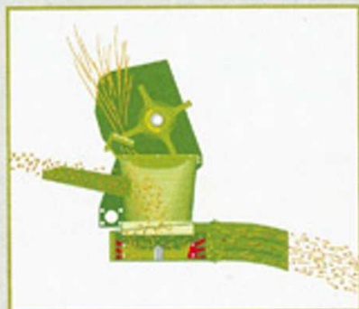
A uniformly short chop. As it leaves the rotors the straw is chopped up, mixed with the chaff and blown onto the field.
